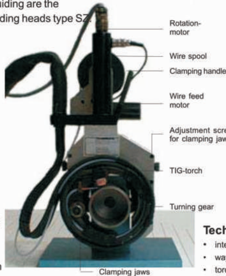
fig.: Orbital-welding head type SZ
