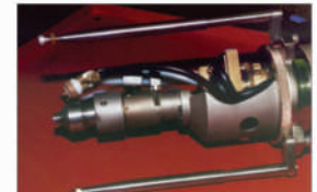
special torch for header drum stud welding
