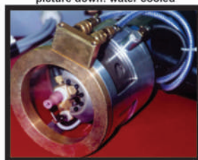
T-250 with double gas shield chamber picture down: water cooled
