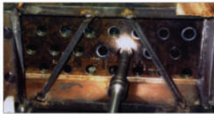
special torch for aircooler tube-tubesheet weldings (2nd tube sheet) Multi pass welding, with filler wire
